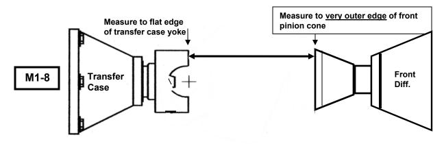
Length from flat edge of transfer case yoke to edge of flange on front differential. Exactly as shown by arrows. Edge to edge only.
